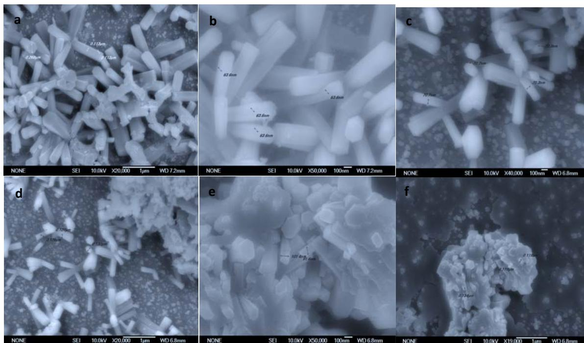
**Figure 1:** FESEM images (top-view) of  $Zn_xCd_{1-x}$  (O) obtained from different compositions of  $ZnCl_2$  and  $CdCl_2$
