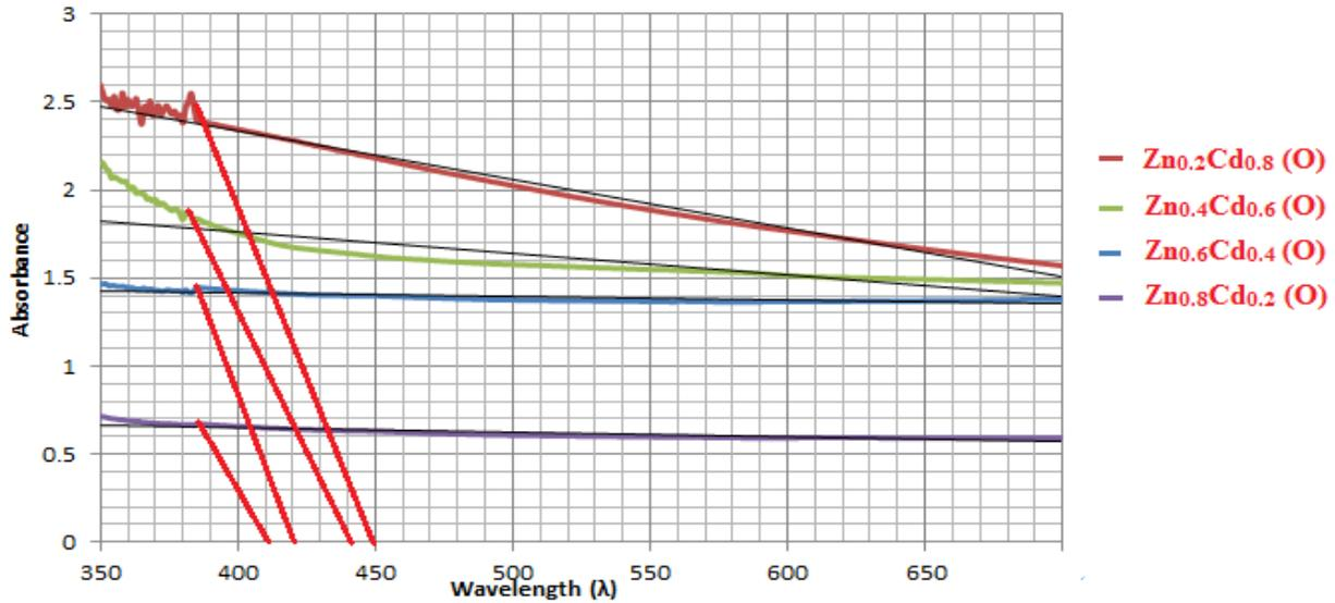
Figure 3: UV visible of  $Zn_xCd_{1-x} (O)$  thin films grown at  $90^\circ C$
