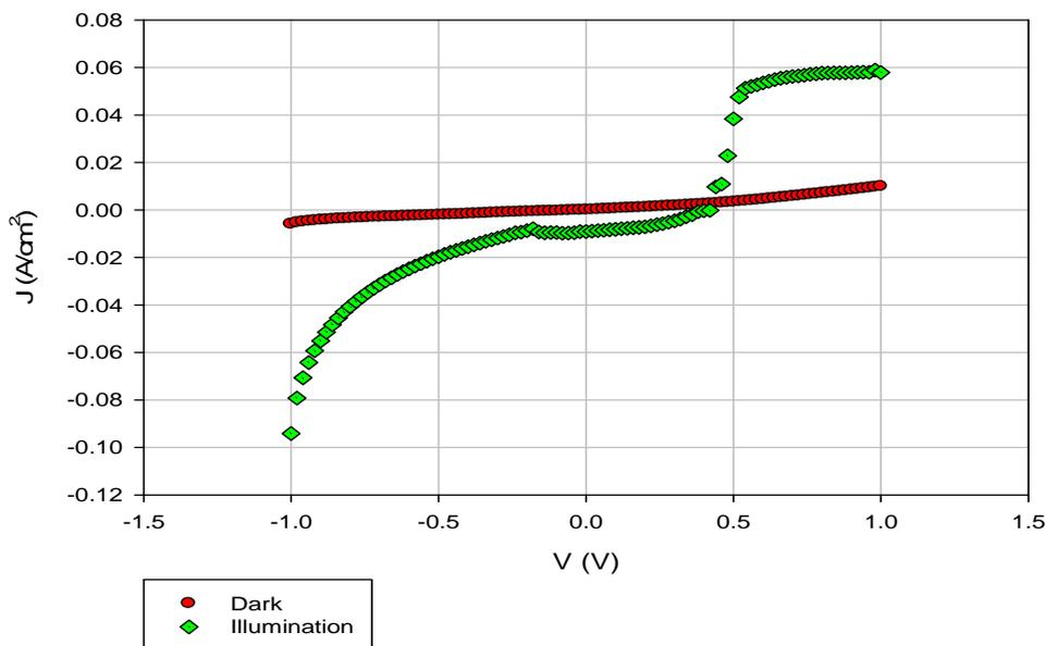
**Figure 4:** Diode like I-V characteristic curve of  $\text{Zn}_{0.6}\text{Cd}_{0.4}$ (O)/PEO + Chitosan in the dark and under illumination condition
