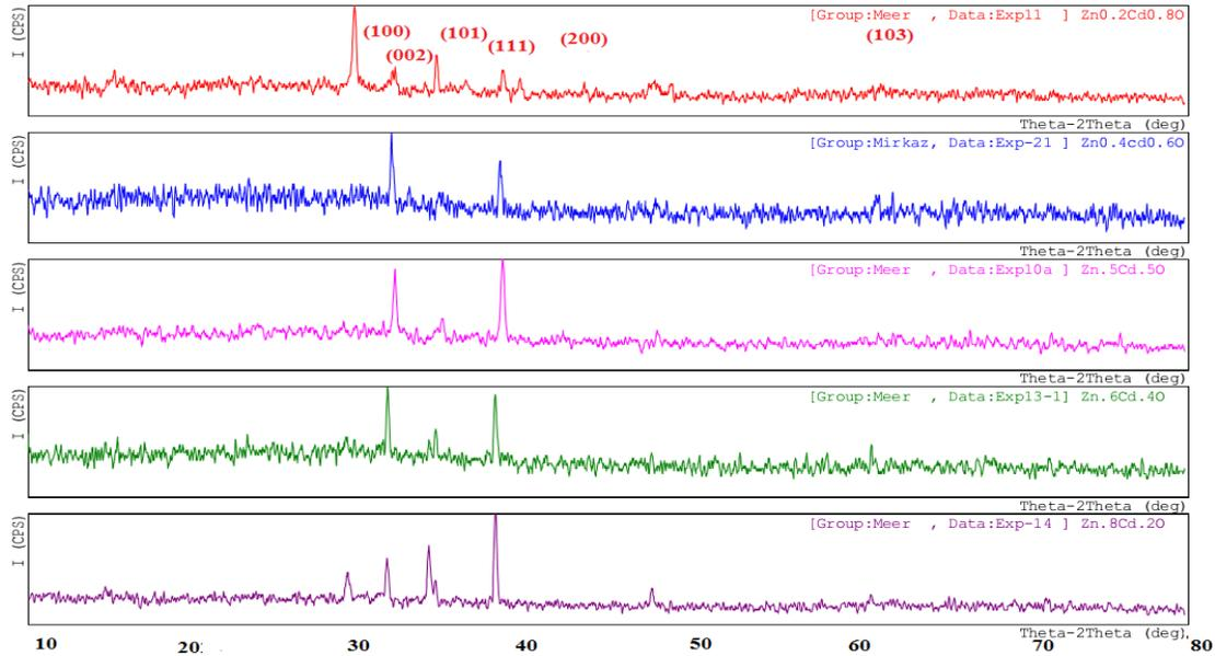
Figure 2: XRD Patterns of  $Zn_xCd_{1-x}O$  thin films on glass substrate deposited at  $90^\circ C$
