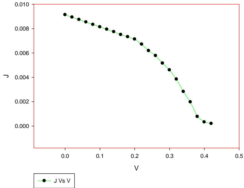
**Figure 5:** Reverse Bias for I-V characterisation of Zn<sub>0.6</sub>Cd<sub>0.4</sub>(O)/PEO + Chitosan under illumination condition
